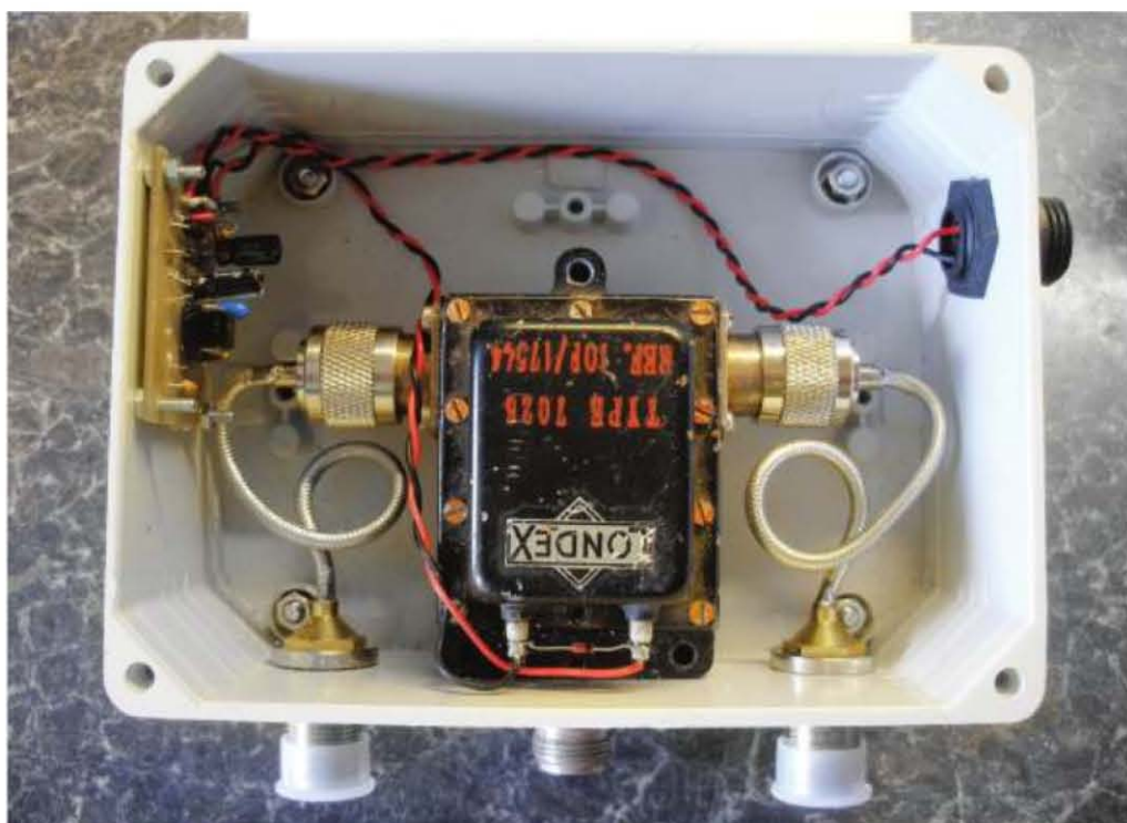
PHOTO 1: The completed masthead unit, with the voltage booster to the left of the central relay.
