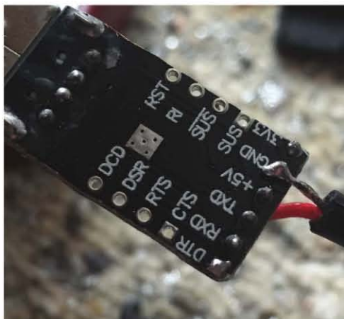
PHOTO 2: The RS-232 pin functions are clearly labelled. The red wire is connected to DTR (on the other side of the board).
