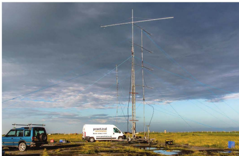
This wonderful aerial system is lots of fun to use on 144MHz - 1 x15 plus 6x4 plus 4x11. Along with quite a bit of sunshine, the team had some torrential showers, one lasting about half an hour, arriving just after kickoff, which made receiving almost impossible due to static rain. Courtesy Gerry, GIORTN.
