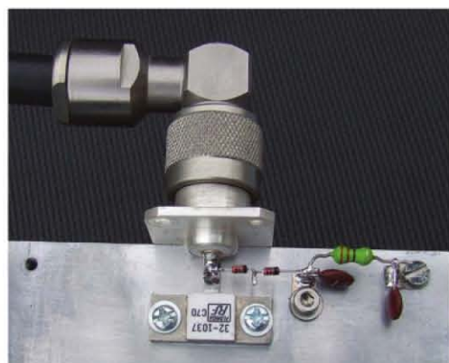
PHOTO 3: 50Ω 250W dummy load and peak detector, usable up to UHF.
