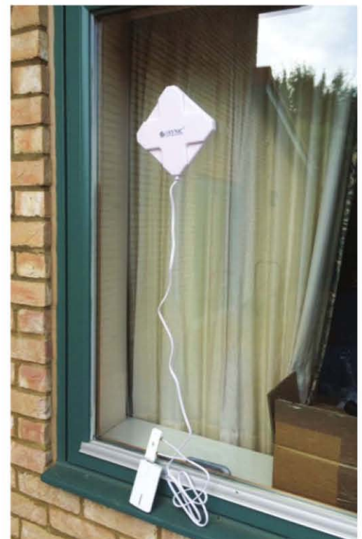
PHOTO 2: Wireless hotspot arrangement. Top to bottom: the eSYNiC antenna, connected to the Huawei 3G/4G dongle that is plugged into the TP Link portable Wi-Fi router.
